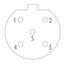
Recommended mating connector type according to IEC 61076-2-10: MM 005-Gx1-B x) A, C, I, P, R or S-type
